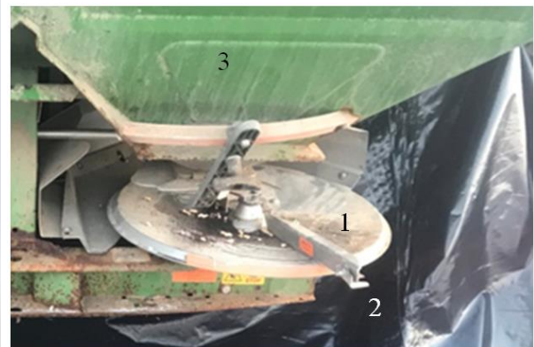
Fig. 4. General view of fertilizer spreader disk, blades and bunker: 1 – the disk, 2 – disk blade and 3 – bunker
